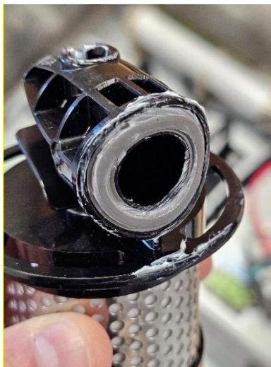
Figure 22: Filter with excessive O-ring lubricant grease
