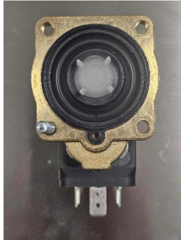
Figure 55: Solenoid diaphragm key hole alignment
