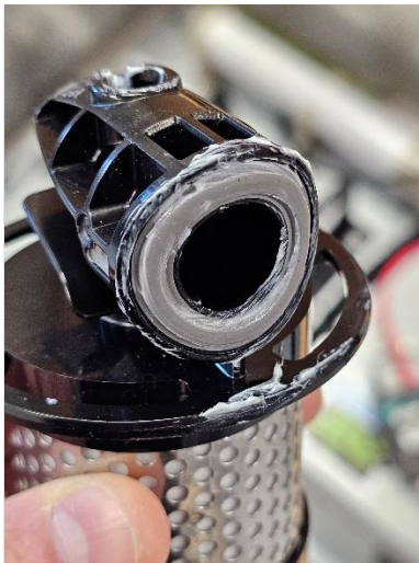
Figure 29: Filter with excessive O-ring lubricant grease
