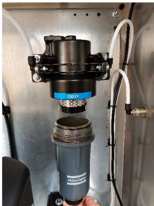
Figure 31: New QD7+ filter inserted
