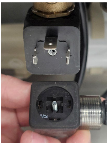
Figure 58: Pin insert alignment for plug and fastener
