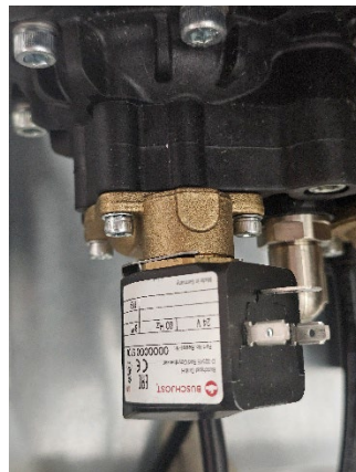
Figure 53: Removing solenoid body fasteners
