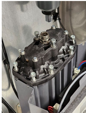
Figure 41: Removing cap fasteners
