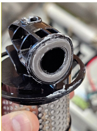
Figure 29: Filter with excessive O-ring lubricant grease
