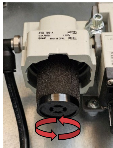
Figure 9: Bowl removed showing old filter
