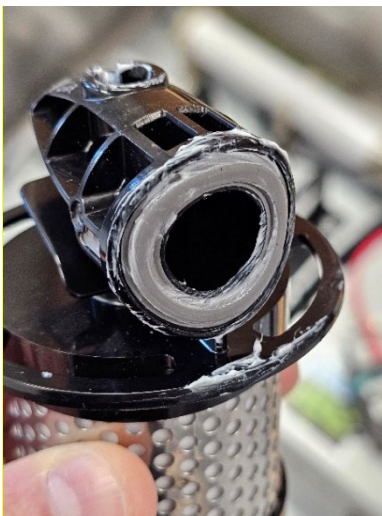
Figure 22: Filter with excessive O-ring lubricant grease
