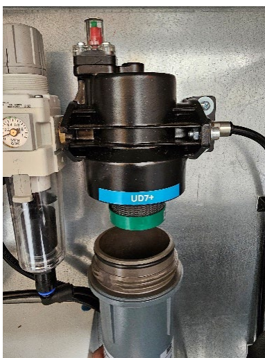
Figure 25: New UD7+ filter inserted
