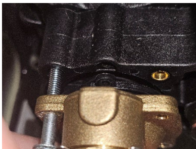
Figure 56: Diaphragm key alignment with housing key way
