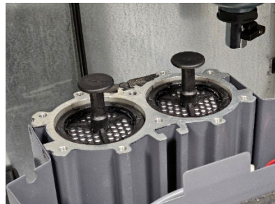
Figure 42: Removed cap reveals desiccant cartridges
