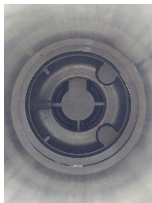
Figure 44: Desiccant chamber cartridge key ways
