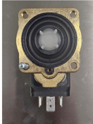
Figure 55: Solenoid diaphragm key hole alignment
