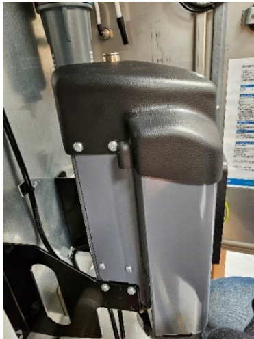
Figure 39: Cover fasteners locations
