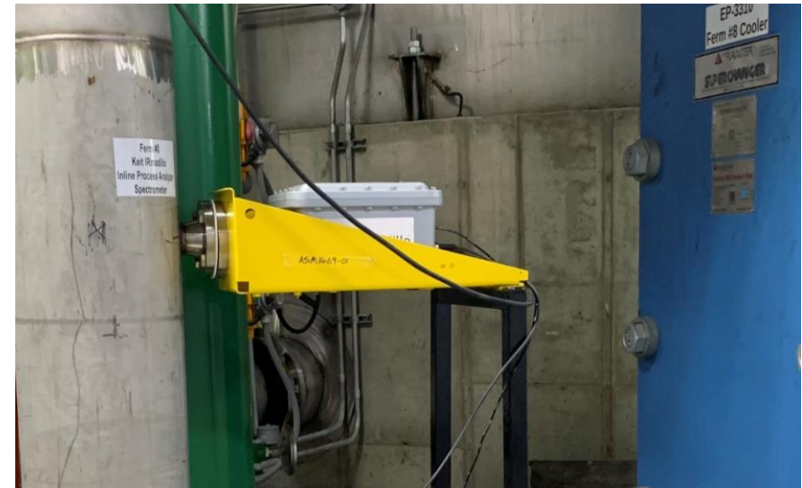
IRmadillo installed directly into recirculation pipe. The cradle allows for easy installation and removal.
