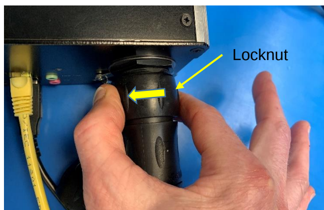
Figure 10: Disconnecting Souriau connectors
