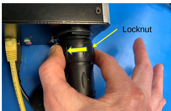
Figure 16: Disconnecting Souriau connectors
