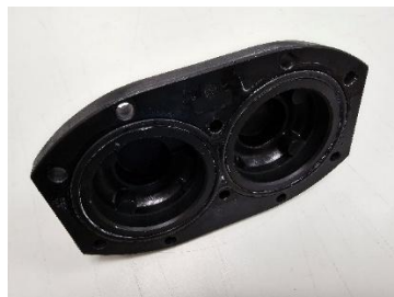
Figure 46: Desiccant chamber cap with new gasket
