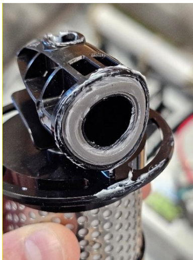
Figure 22: Filter with excessive O-ring lubricant grease
