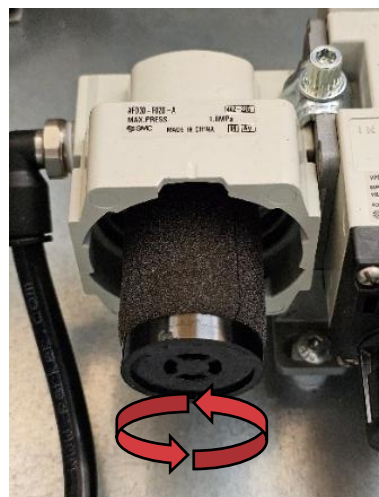
Figure 9: Bowl removed showing old filter
