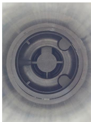
Figure 44: Desiccant chamber cartridge key ways
