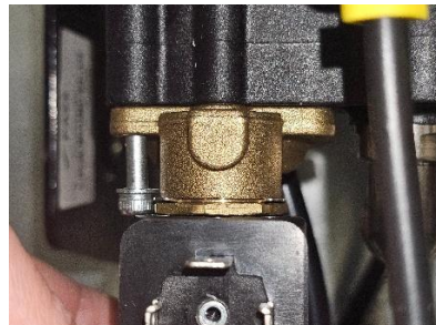
Figure 57: Solenoid seated without gap or diaphragm pinching
