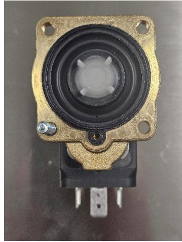
Figure 55: Solenoid diaphragm key hole alignment
