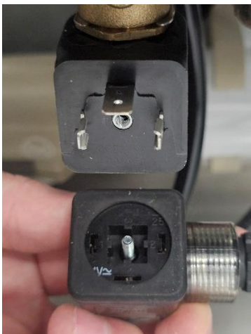
Figure 58: Pin insert alignment for plug and fastener
