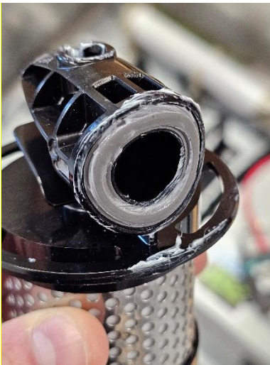
Figure 29: Filter with excessive O-ring lubricant grease
