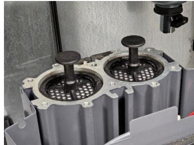
Figure 42: Removed cap reveals desiccant cartridges
