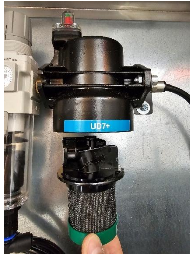
Figure 24: Inserting new UD7+ filter
