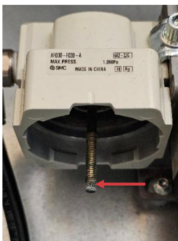
Figure 10: Old filter removed to reveal threaded core fastener
