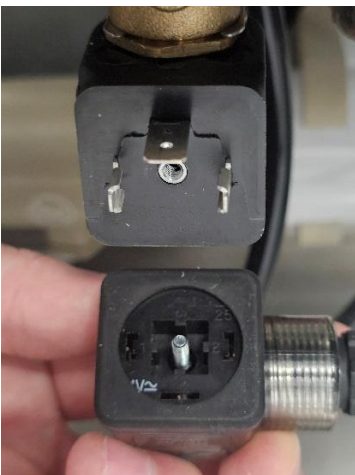
Figure 58: Pin insert alignment for plug and fastener
