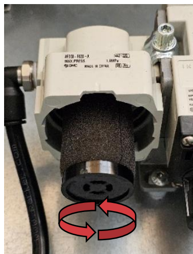
Figure 9: Bowl removed showing old filter
