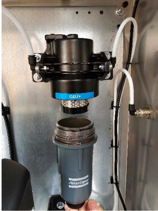
Figure 31: New QD7+ filter inserted
