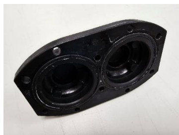
Figure 46: Desiccant chamber cap with new gasket
