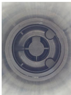
Figure 44: Desiccant chamber cartridge key ways
