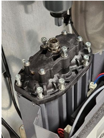
Figure 41: Removing cap fasteners
