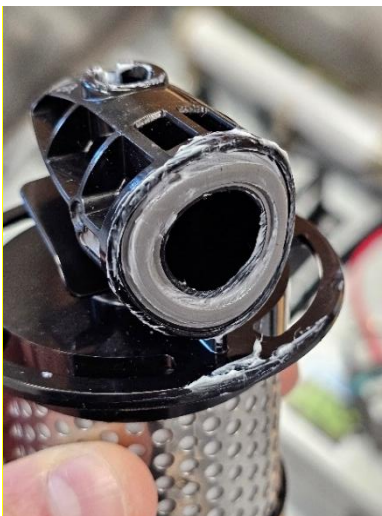
Figure 22: Filter with excessive O-ring lubricant grease
