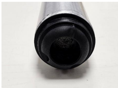
Figure 45: Cartridge reciprocal keys
