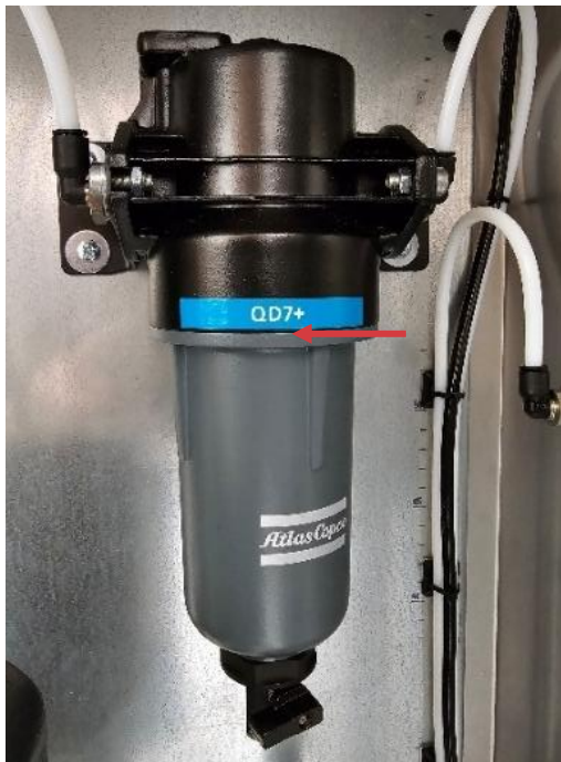
Figure 32: Filter bowl fastened with no gap at seam
