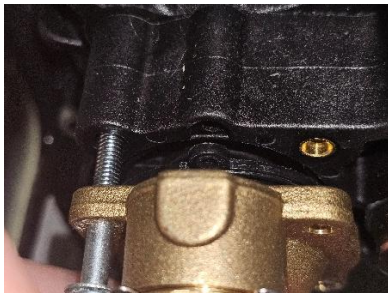
Figure 56: Diaphragm key alignment with housing key way
