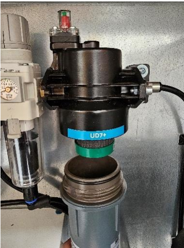
Figure 25: New UD7+ filter inserted
