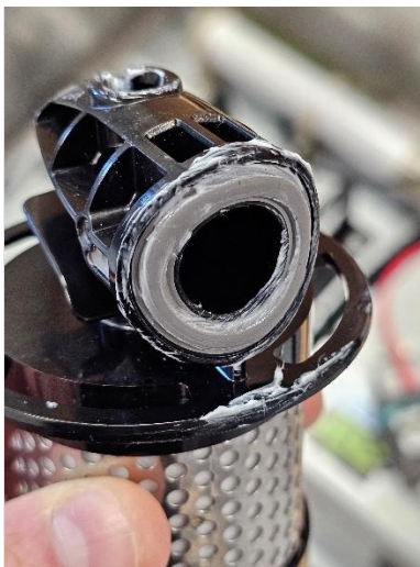
Figure 29: Filter with excessive O-ring lubricant grease
