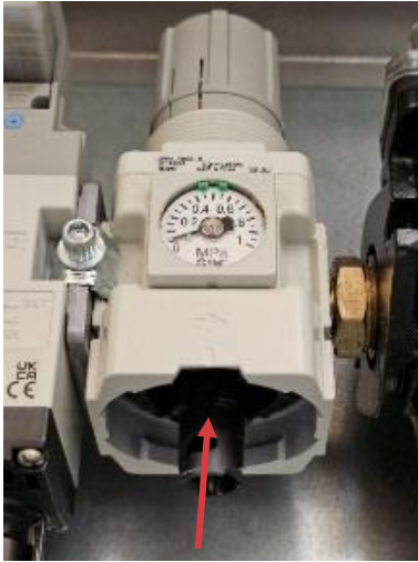
Figure 17: Female bayonet reciprocal on SMC AW30
