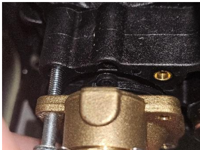
Figure 56: Diaphragm key alignment with housing key way
