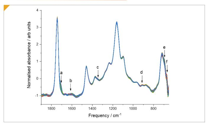
Figure 1: Example spectra of a mixture of triglyceride feedstocks. Band assignment: a) C=O in FFAs, b) C=C bonds in unsaturated FFAs and FAMEs, c) C-H bends in FFAs and FAMEs, d) C-C and C-O stretches in FFAs and FAMEs, e) O-C=O bend in FFAs, f) O-C=O bends in FFAs and FAMEs
