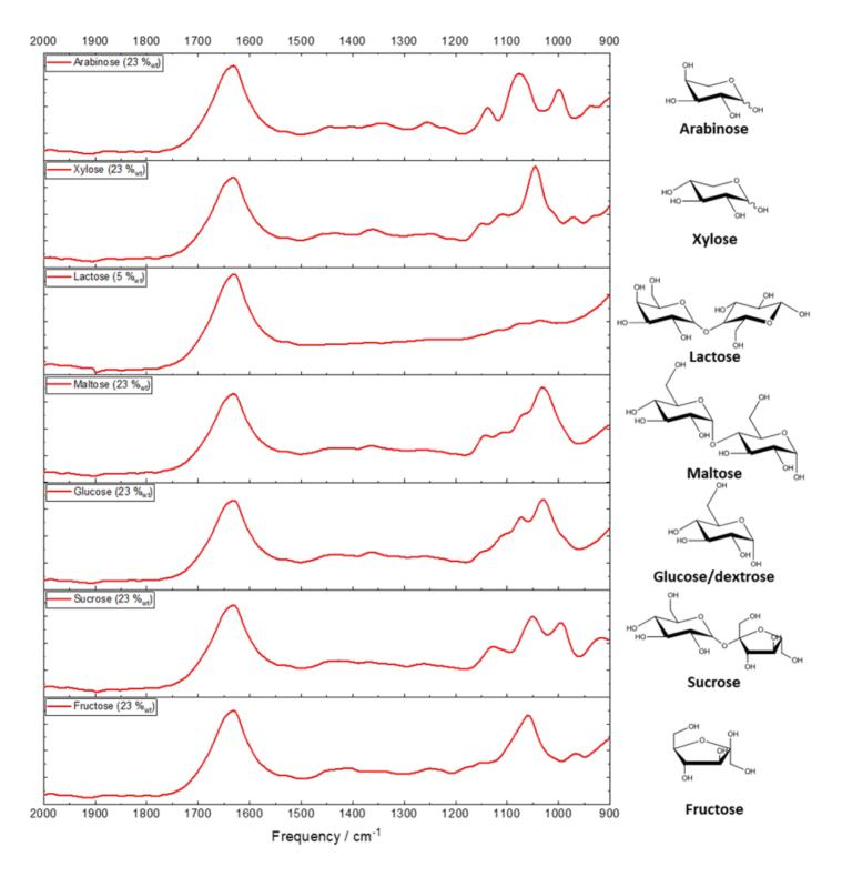
**Figure 2:** Spectra of seven sugar solutions acquired on an IRmadillo with a 120 s sampling time between 900 and 2000 cm<sup>-1</sup>. The structures of the sugars are shown to the right.
