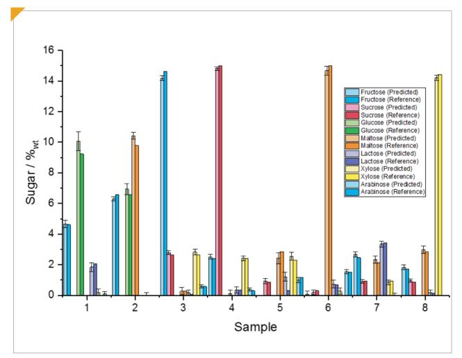
Figure 3: Predictions for mixtures of sugars using the IRmadillo and a pre-built PLS model.
